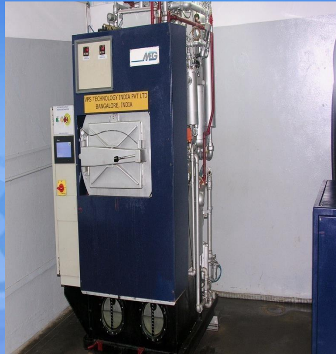
Vapor degreasing machine
